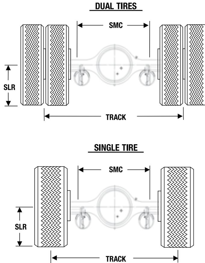
**TRACK** – The distance between the dual tire centerlines or the distance between the tire centerlines on a single tire.
