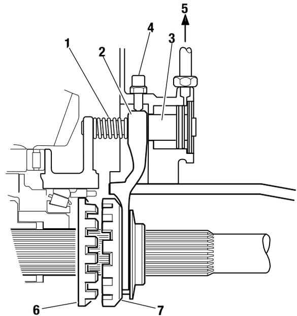
**Differential Lock Disengaged**
